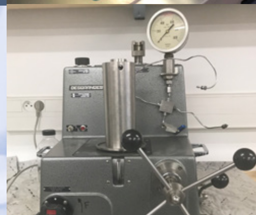
Strength (with dynamometer) & pressure (with deadweight tester)
