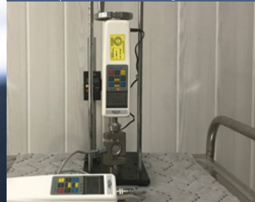
Strength (with dynamometer) & pressure (with deadweight tester)
