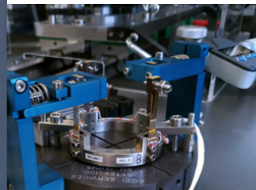
Extensometers calibration & expansion ring calibration
