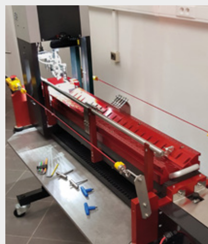
Field mobile Rock-testing facility "Micro-indentation" device to determine the mechanical properties on the surface of a full diameter core.
